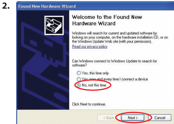
2. The New Hardware Wizard automatically appears. Select <No, not this time> and click <Next>.
