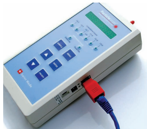
ParticleScan with crossover adapter and patch cable for direct connection into the RJ-45 network connector of a computer.
